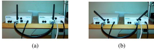
Fig. 22. Polarization of the receive antennas; (a) vertically polarized, (b) perpendicular angled at 45°.
