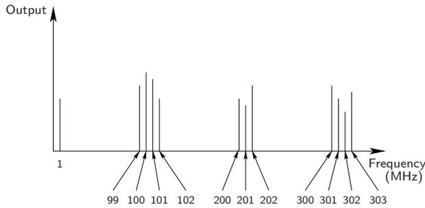
Fig. 3: Output spectrum from a two-tone signal applied to a 3rd order non-linear system
