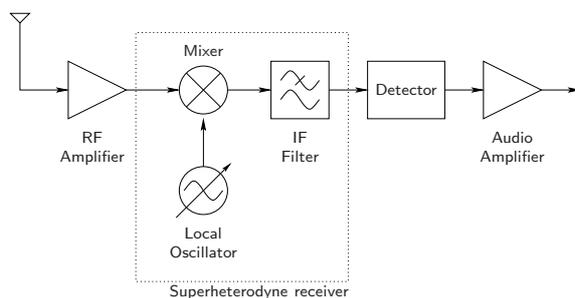
Fig. 1: Block diagram for a superheterodyne receiver.
