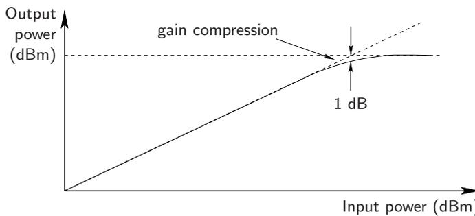
Fig. 4: Gain compression for an amplifier.
