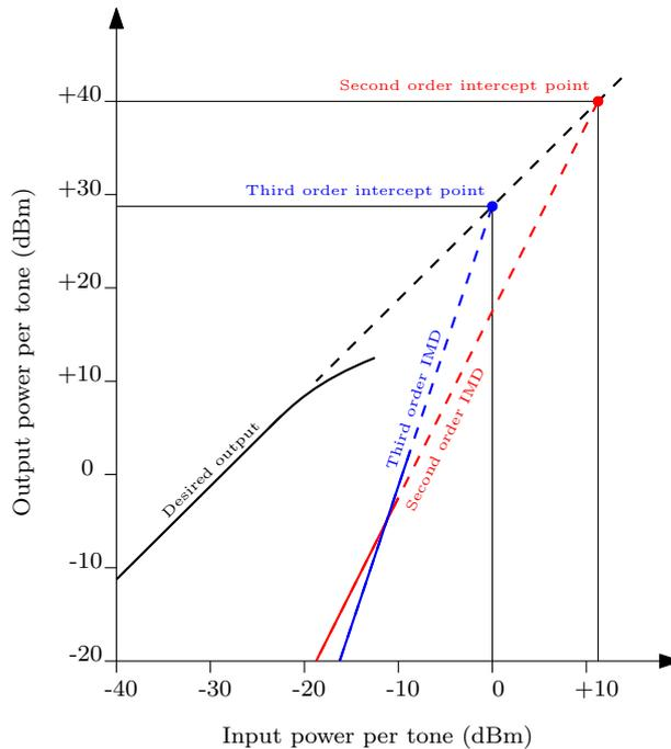
Fig. 5: Second and third order intercept points for an RF amplifier (what is the gain of this amplifier?)
