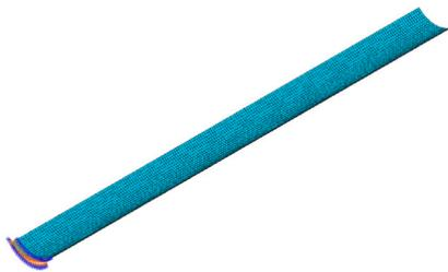
**Fig. 5.** Deployed frequency analysis of the shell with a boundary condition fixed in the 6 Degree Of Freedom (DOF).
