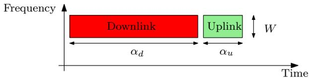
Fig. 1. Allocation of up-link and down-link channels for time-division duplexing (TDD). For asymmetric scenarios, TDD can allocate a larger proportion of the frame to the high-rate link.
