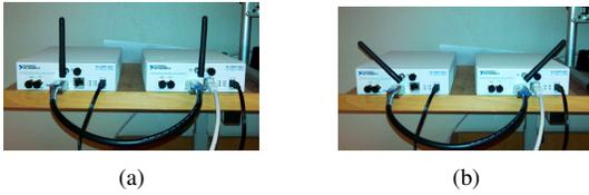
Fig. 22. Polarization of the receive antennas; (a) vertically polarized, (b) perpendicular angled at  $45^\circ$ .
